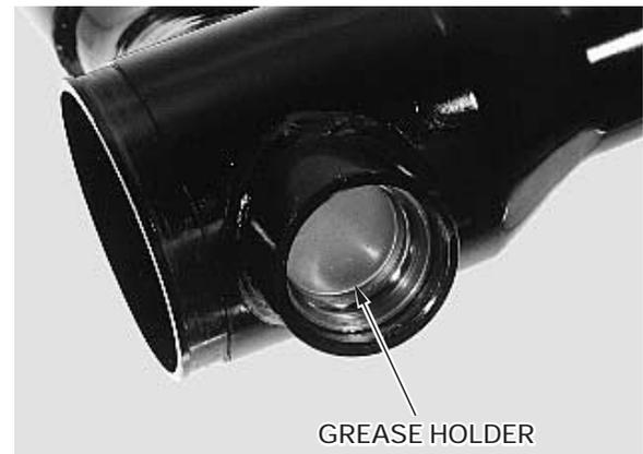
Pull the outer race out of the swingarm using a commercially available 3/8 in × 16 sliding hammer and the special tool.
