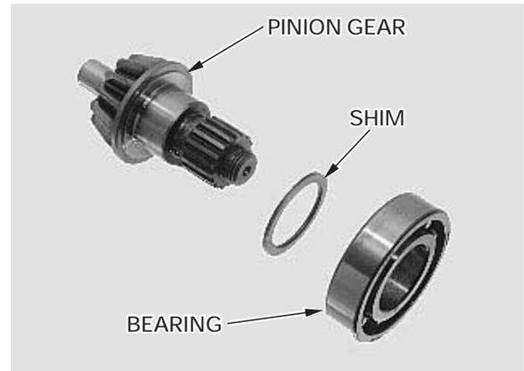
Drive the bearing with the marking side facing up.
