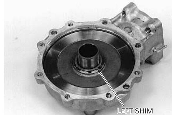
*It is important to turn the pinion while tightening the bolts. If the ring gear shim is too thick, the gears will lock after only light tightening.*
