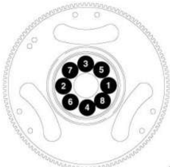
Fig. 212: Flex Plate Tightening Sequence Courtesy of CHRYSLER GROUP, LLC
