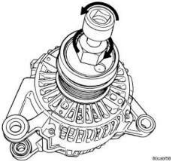
Fig. 18: DECOUPLER INSTALLATION (Litens) Courtesy of CHRYSLER LLC
